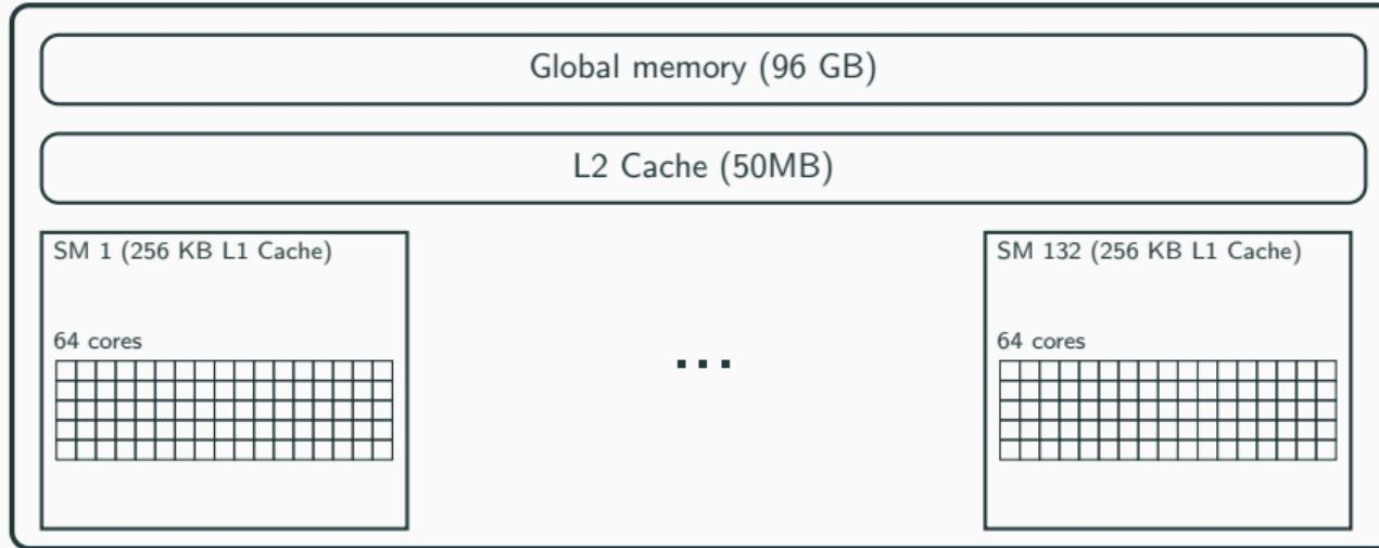
**8448 cores grouped in 132 streaming multiprocessors (SM) of 64 cores each (H100).**
